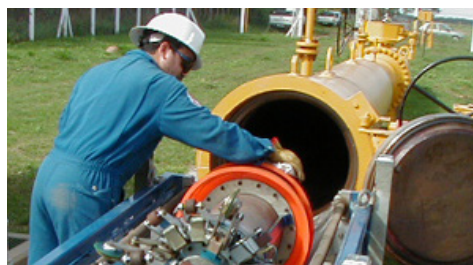
Pipeline inspection gauges require inertial navigation and positioning data from KVH inertial sensors to accurately maneuver through miles of underground pipeline where GPS/GNSS signals cannot be received.
